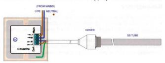
250 watt element fitted into your Towel Rail, then **1 lit red 'LED' IN THE SET OF 5**, will mean that you are using 50 watts of power, 2 led's means 100 watts etc up to full power of 5 LED's, using 250 watts.
